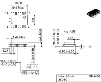
\*Dimension including the plating thickness
