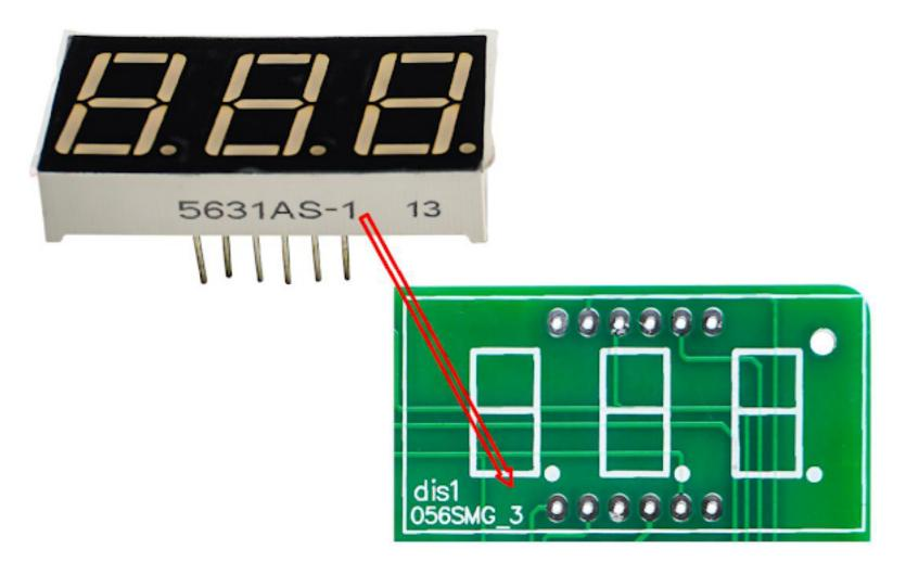
The model number is marked on one side of the digital tube, and the model number is also marked on the bottom.
