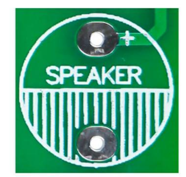
The passive buzzer does not distinguish between positive and negative poles, install it in the SPEAKER position.
