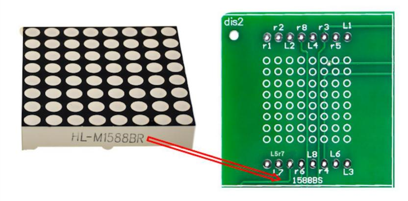
The model number is marked on one side of the 1588 dot matrix screen, and the model number is also marked on the bottom. According to the model mark on the silk screen, install the dot matrix screen to the dis2 and dis3 positions respectively.
