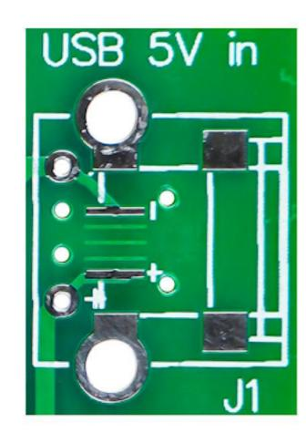
Install the USB socket to the J1 position with the socket facing outward. When soldering, you need to preheat the pins of the shell and use more solder to solder it firmly.
