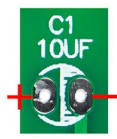
The short pin of the electrolytic capacitor is the negative electrode, and the negative electrode side is printed with white paint. The silk screen also has white paint printed on the negative electrode side. The polarity must be matched during installation. The 10uF electrolytic capacitor is installed horizontally at position C1.
