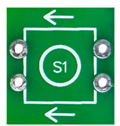
The tactile switch does not distinguish polarity and is installed in the S1-S5 position.
