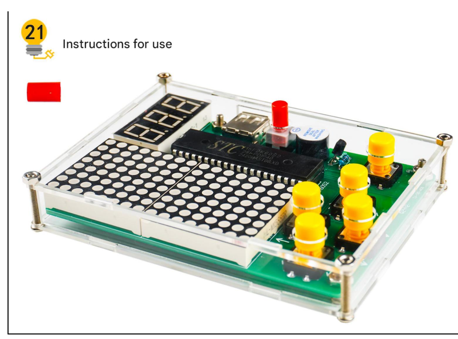
Install the red power button cap on the self-locking switch to complete the final assembly of the game console. After turning on the power, press the red button to turn on the game console.
