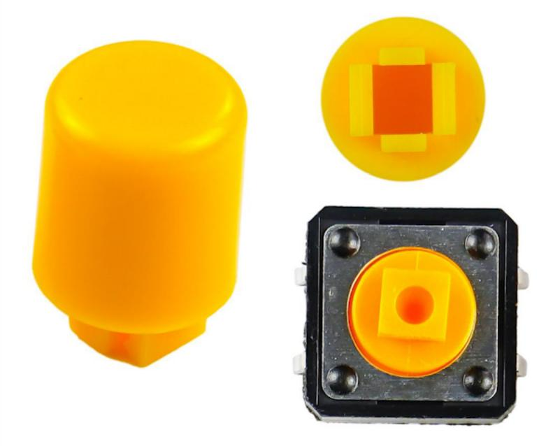
Install the button caps onto the 5 tact switches respectively.
