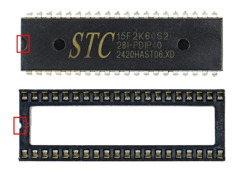
There is a gap on one side of the microcontroller, and the IC holder also has a gap for corresponding installation.
