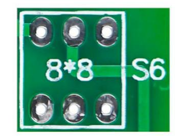
The self-locking switch is installed in the S6 position with the strip-shaped
