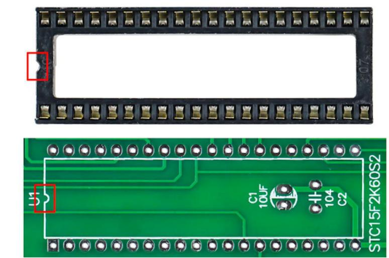
There is a notch on one side of the IC holder, and its silk screen also has a notch, corresponding to the U1 position.
