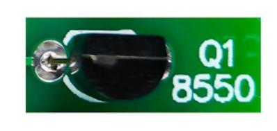
The cross-section of the 8550 transistor is horseshoe-shaped.
