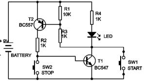
point on, both transistors keep each other in conducting state, even when the "START" button is released. Pressing the "STOP" button will end the current flow towards the base of T1 and it will stop conducting. The circuit is interrupted and T2 will also stop conducting. The LED will turn off.
