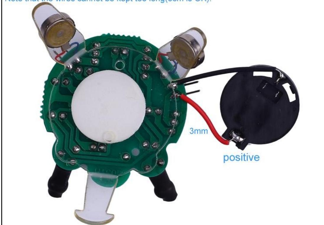
Step 23: Paste CR2032 Battery Socket onto PVC bracket with a Double Sided Adhesive Tape.
