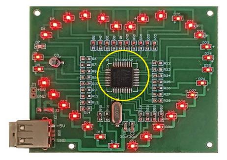
6. Solder the IC Chip into position. Make sure the dot at the corner of the chip matches the notch marking on the circuit board.
