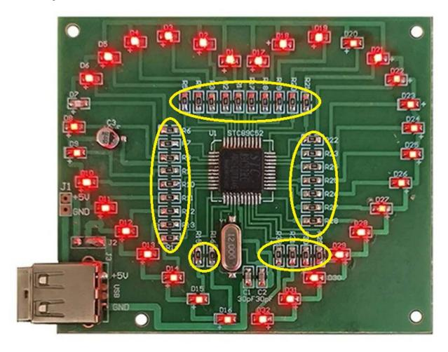
1. Solder the 560 Ohm SMD Resistors into locations R1 to R32 marked 561. Polarity does not matter.
