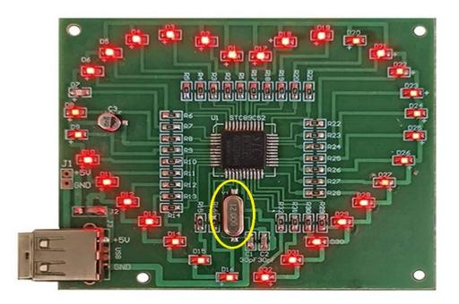
5. Solder the crystal oscillator into place. Polarity does not matter.
