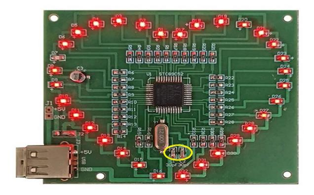
2. Solder the 30pf SMD Capacitors into locations C1 and C2 marked 300. Polarity does not matter.
