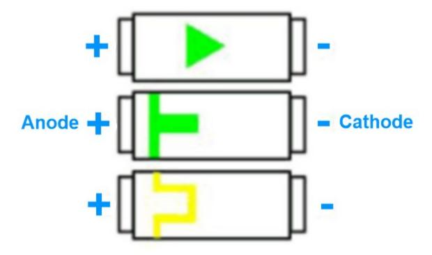
4. Solder the SMD LEDs into the locations D1 to D32. Pay attention to the polarity and place the positive side where the + is marked on the board.
