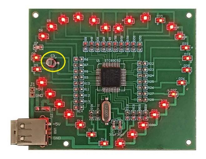
3. Solder the 10uf SMD Capacitor into location C3. Pay attention to the polarity so the + side is in the correct location according to the silkscreen on the PCB.
